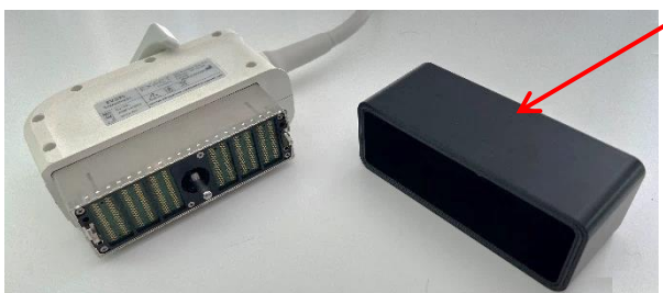
Figure 32: Lockable Transducer Connector Cover
