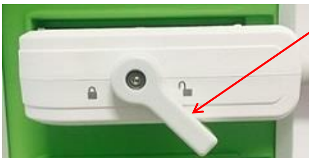
Figure 30: Unlocked Transducer Connector Lock Knob
