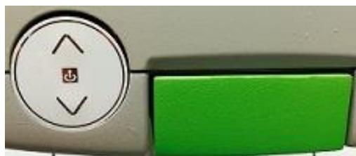
Figure 10: Control Panel/Monitor Height
