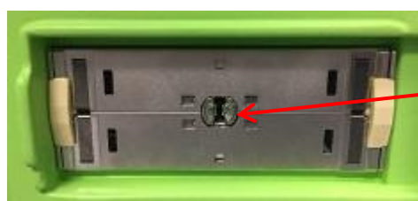
Figure 20: Lock Notch on the Transducer Connector Slot
