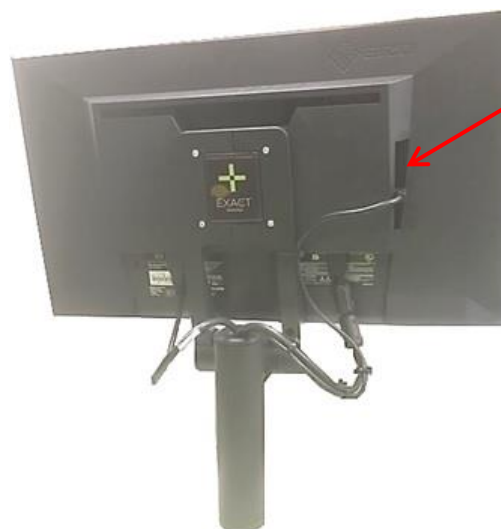
Figure 8: USB Connectors on the Rear of the Monitor (available in some ExactVu system configurations)
