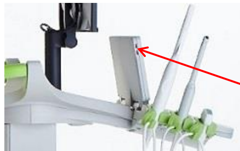
Figure 7: USB Connectors on the Left Side of the Touch Screen
