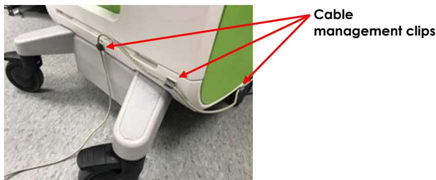
Figure 4: Foot Pedal Cable Management
